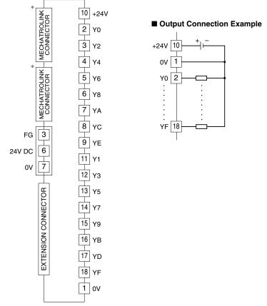
\*MECHATROLINK connectors are internally connected. The network cable can be connected to either one.
