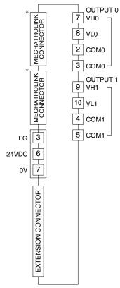
\*MECHATROLINK connectors are internally connected. The network cable can be connected to either one.
