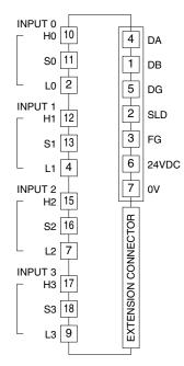
In order to improve EMC performance, bond the FG terminal to ground. Caution: FG terminal is NOT a protective conductor terminal.
