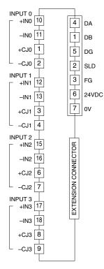
In order to improve EMC performance, bond the FG terminal to ground. Caution: FG terminal is NOT a protective conductor terminal.
