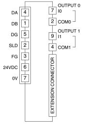
In order to improve EMC performance, bond the FG terminal to ground. Caution: FG terminal is NOT a protective conductor terminal.
