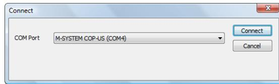
Click [Monitor] button to open the COM Port dialog box. Specify the COM port and click [Connect] to open the COM port. When the communication is established, the following window appears on the screen.
