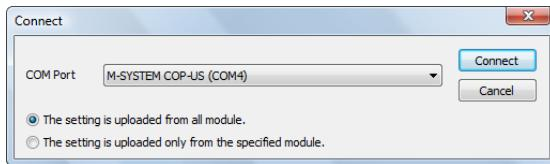
Choose the COM port number to which the device is connected with the PC Configurator Cable. The port number depends on the PC. Choose an adequate port.
