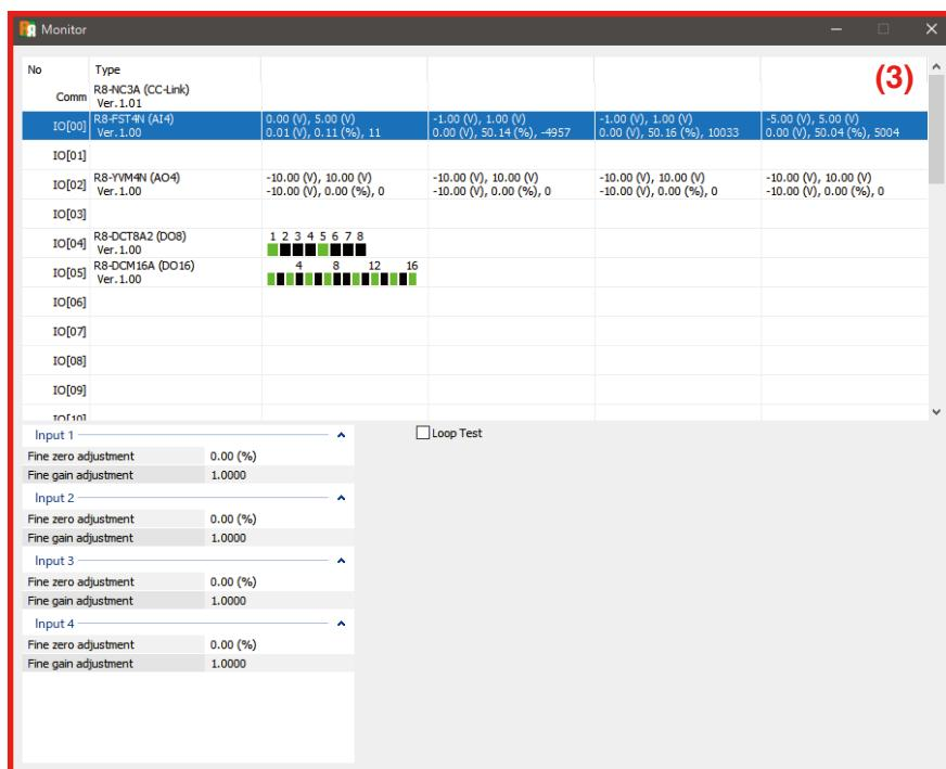
Monitor view shows all the connected modules and their I/O status on the upper window.
