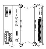
Confirm that the locking clamps of the I/O module are set. Insert the module in parallel to the next one while aligning the grooves of both modules (A & B in the above figure).
