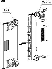
The protective cover is to be attached over the connected I/O module at the right end.
