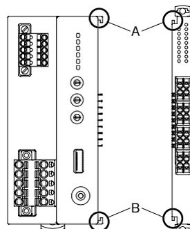
Confirm that the locking clamps of the I/O module are set. Insert the module in parallel to the next one while aligning the grooves of both modules (A & B in the above figure). Maintain it perpendicularly to the rail.
