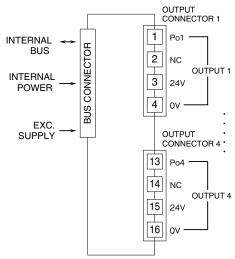
Note: Pin 3, 7, 11 and 15 of output connector are connected to 24V of the excitation supply. Pin 4, 8, 12 and 16 of output connector are connected to 0V of the excitation supply.
