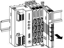
• Removing an intermediate module
