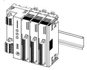
When removing the cover, pull it out while squeezing the hooks inward.
