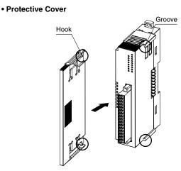
The protective cover is to be attached over the connected  $\ensuremath{\mathsf{I/O}}$  module at the right end.
