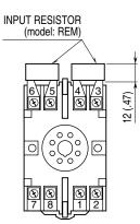
Input shunt resistor attached for current input.
