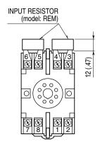
Input shunt resistor attached for current input.
