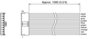
\* One end of the cable is cut off.
