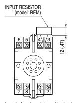
Input shunt resistor attached for current input.
