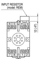
Input shunt resistor attached for current input.
