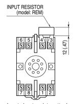
Input shunt resistor attached for current input.
