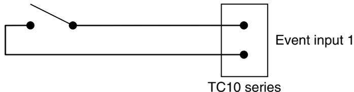
2. Specify event input assignment and temperature setpoint in switching to the bank 2.
