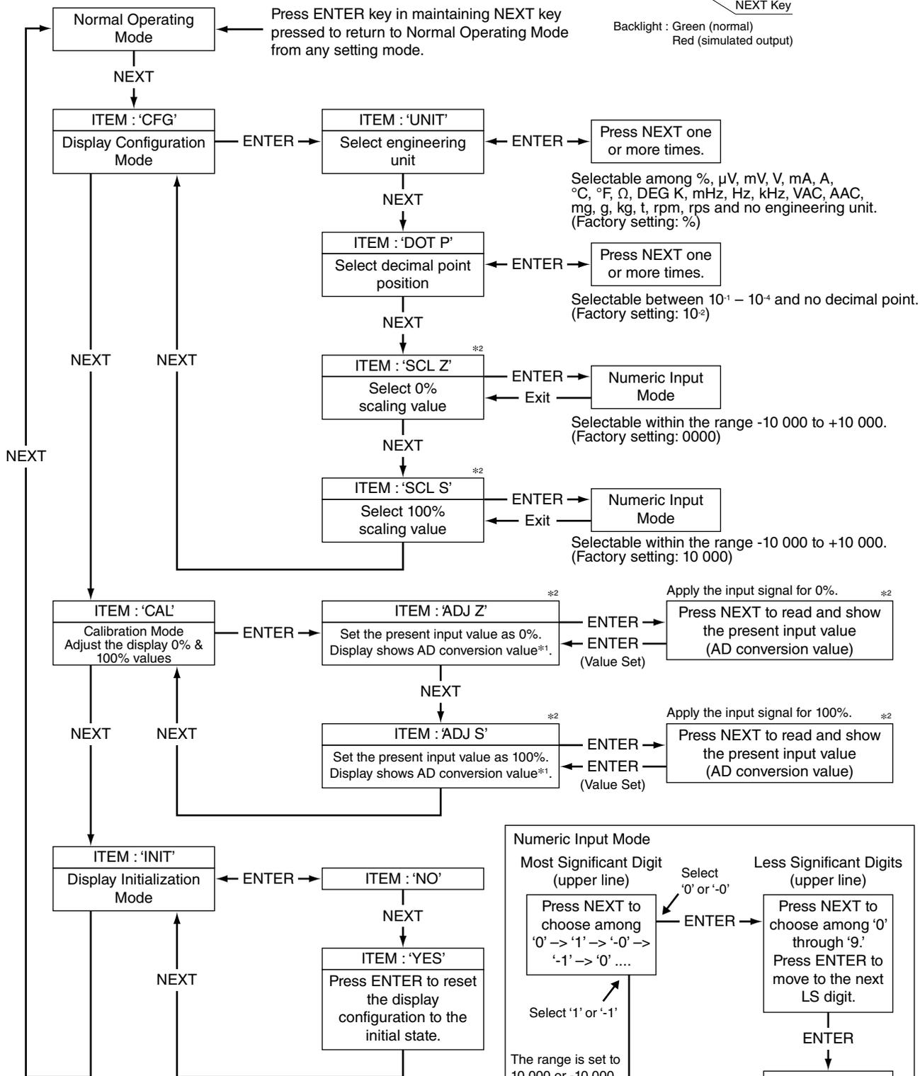
\*1. 'AD conversion value' means the internal digital data representing the input signal, which is computed to a percentage. It is not a % or engineering unit value.
