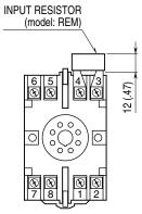
Input shunt resistor attached for current input.
