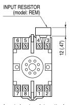
Input shunt resistor attached for current input.
