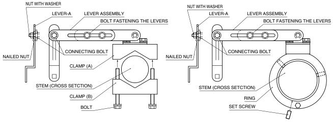
Figure 1. ATTACHING THE VOLK-A, B, B1 (VOLK shapes are slightly different between different suffix code types.)
