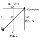
6) Input 0%, 50% and 100% signals and check the output according to the respective input value. If the output value is shifted, repeat the above procedure (2) - (5).
