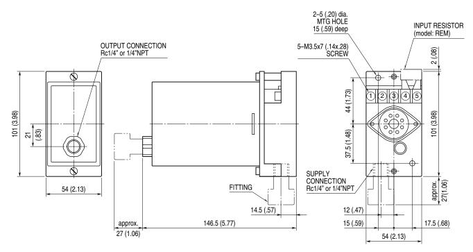
•When mounting, no extra space is needed between units. •Fittings are provided for 1/4"NPT connection.
