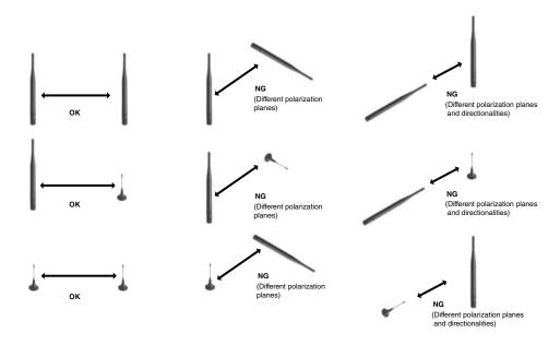
Figure 9.1 Polarization plane of antenna
