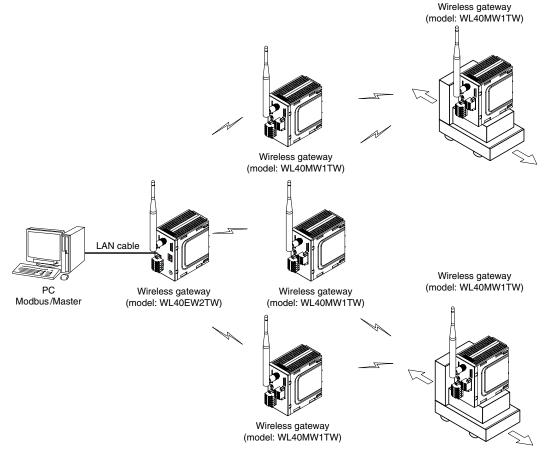
Figure 1.2 System configuration example including low-speed moving device
