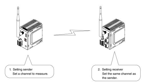
Figure 6.15 Configuration of communication test
