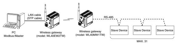
Figure 1.1 System configuration example
