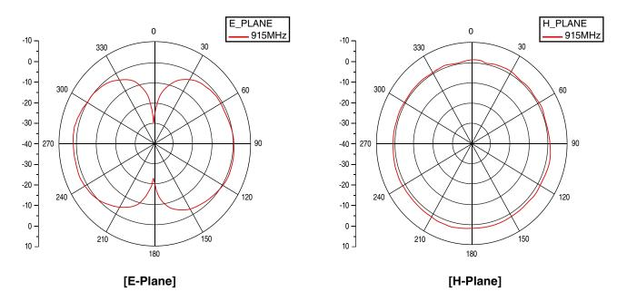
Figure 9.2 Directionality of sleeve antenna for WL40TW series <reference>
