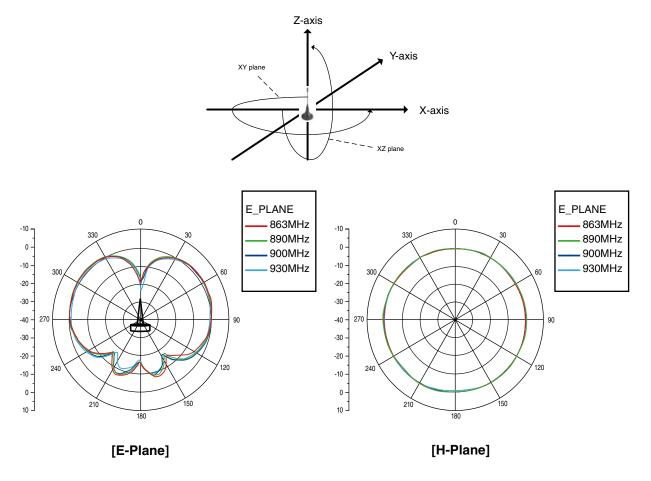
Figure 9.3 Directionality of rooftop antenna for WL40TW series <reference>
