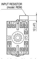
Input shunt resistor attached for current input.
