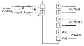
\*Input shunt resistor attached for current input.
