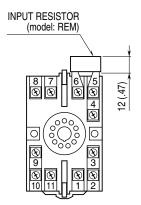
Input shunt resistor attached for current input.
