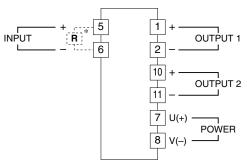
\*Input shunt resistor attached for current input.
