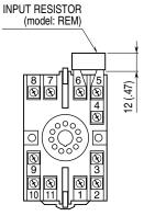
Input shunt resistor attached for current input.
