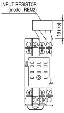
Input shunt resistor attached for current input.
