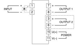
The section enclosed by broken line is only with 2nd output option. \*Input shunt resistor attached for current input.
