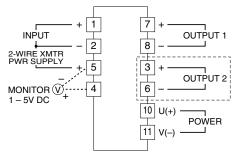
The section enclosed by broken line is only with 2nd output option.
