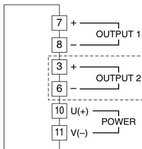
The section enclosed by broken line is only with 2nd output option.
