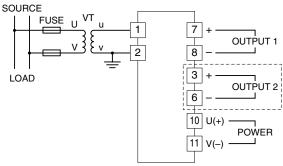
The section enclosed by broken line is only with 2nd output option.
