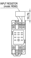
Input shunt resistor attached for current input.
