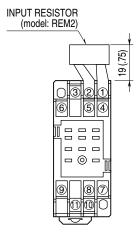
Input shunt resistor attached for current input.
