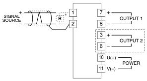
\*Input shunt resistor attached for current input.
