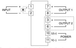
The section enclosed by broken line is only with 2nd output option. \*Input shunt resistor attached for current input.
