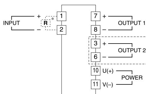
The section enclosed by broken line is only with 2nd output option.
