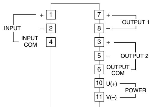
Note: The section enclosed by broken line is only with 2nd output option.
