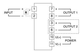
The section enclosed by broken line is only with 2nd output option. \*Input shunt resistor attached for current input.
