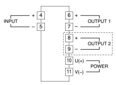
The section enclosed by broken line is only with 2nd output option.
