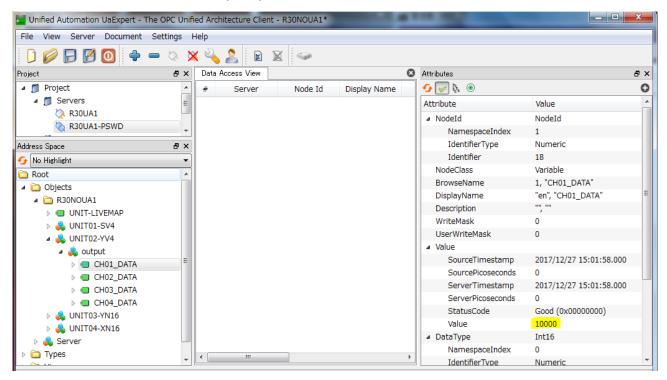
In this example, the value '10000' is written in CH01\_DATA in INT16 form, indicating that the YV4 module outputs 100.00% from CH01.
