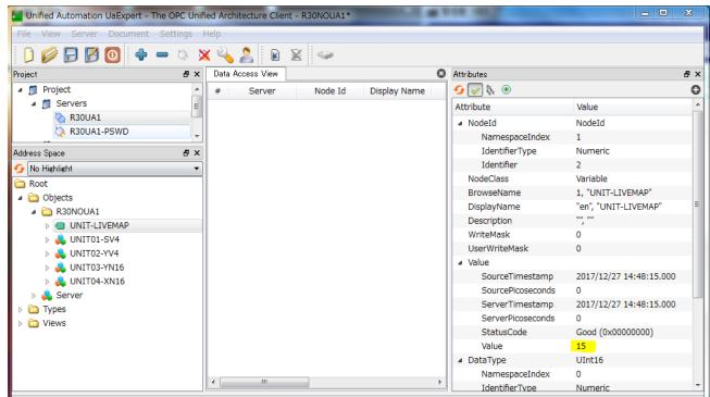
In this example, the value of UNIT\_LIVEMAP is '15 (000FH)', indicating that I/O modules are mounted in the slot Nos. 1 through 4.
