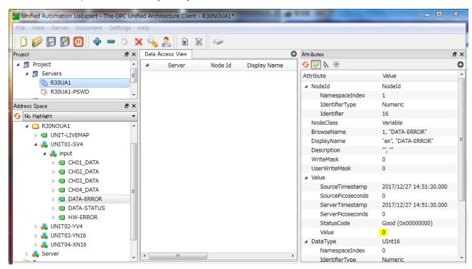
In this example, the value of DATA-ERROR is '0 (0000H)', indicating that the input values of CH01 to CH04 are normal.
