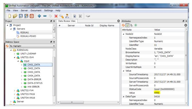
In this example, the value of CH01\_DATA of the SV4 module is '4999' in INT16 form, indicating that the input value of CH01 is 4999.
