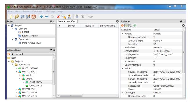
In this example, the value '196608 (30000H)' is written in CH01\_DATA in UINT32 form to allocate presetting bits, thereby setting 30000 as the preset count value for the PA2 module.
