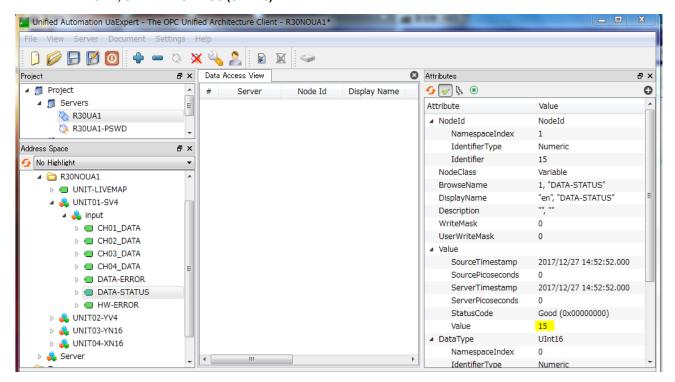
In this example, the value of DATA-STATUS is '15 (000FH)', indicating that the input values of CH01 to CH04 are valid.
