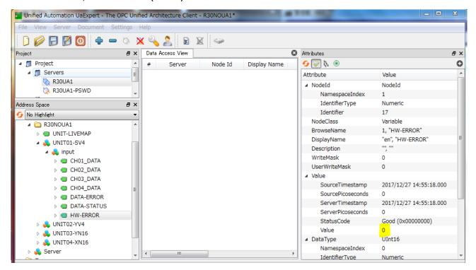
In this example, the value of HW-ERROR is '0 (0000H)', indicating that no HW error is occurring on CH01 to CH04.
