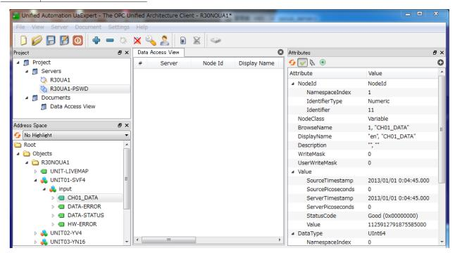
In this example, the value of CH01\_DATA of the SVF4 module is '1125912791875585000 (0FA0 0BB8 07D0 03E8H)' in UINT64 form, indicating that the values of CH01, CH02, CH03, and CH04 are '03E8H', '07D0H', '0BB8H', and '0FA0H', respectively.
