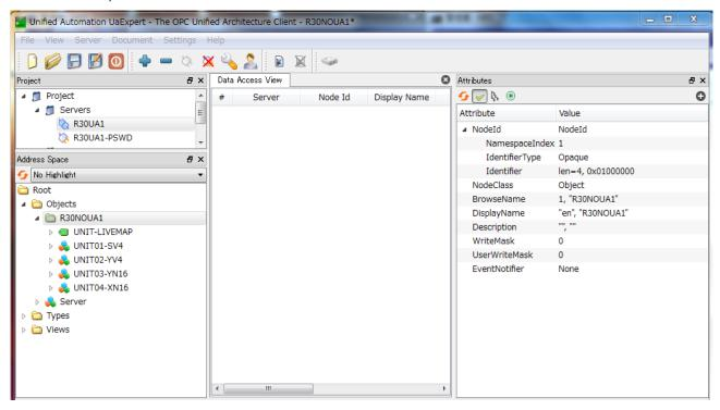
Object nodes of respective I/O modules which are detected at power up and a variable node indicating I/O module status (UNIT\_LIVEMAP) are created in the address space of R30NOUA1.
