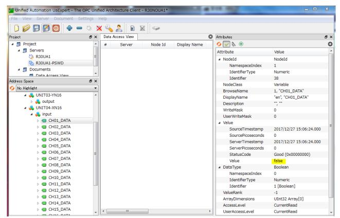
In this example, the value 'false' is written in CH01\_DATA in BOOLEAN form, indicating that input of CH01 of the XN16 module is OFF.
