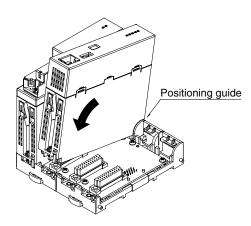
3) Tighten the base fixing screw using a screwdriver (stem length: 70 mm/2.76" or more) (torque 0.5  $N\!\cdot\!m).$
