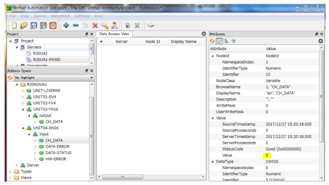
In this example, the value (0.0000H) is written in CH\_DATA in UINT16 form, indicating that inputs of all channels of the XN16 module are OFF.
