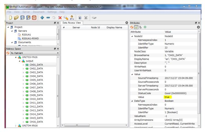
In this example, the value 'true' is written in CH01\_DATA in BOOLEAN form, indicating that output of CH01 of the YN16 module is ON.
