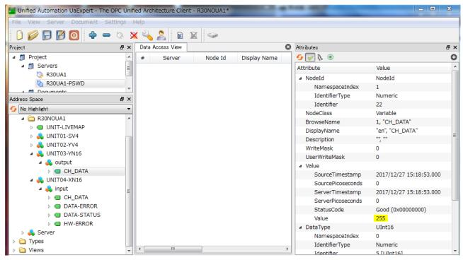
In this example, the value '255 (00FFH)' is written in CH01\_DATA in UINT16 form, indicating that outputs of CH01 to CH16 of the YN16 module are ON.
