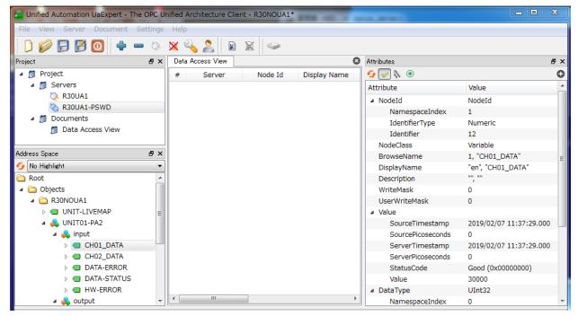
In this example, the value of CH01\_DATA of the PA2 module is '30000' in UINT32 form, indicating that the value of the totalized pulse count of CH01 is 30000.
