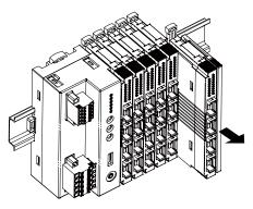
• Removing an intermediate module
