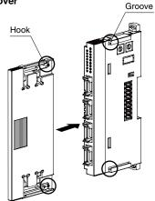
The protective power is to be attached over the connected I/O module at the right end.
