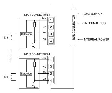
Note: For dry contact input, connect it across the terminals 3 and 4.
