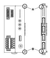
Confirm that the locking clamps of the I/O module are set. Insert the module in parallel to the next one while aligning the grooves of both modules (A & B in the above figure).
