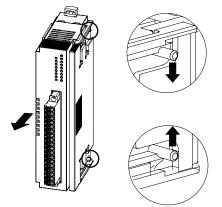
■ HOW TO UNMOUNT THE MODULE FROM DIN RAIL
