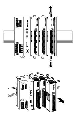
• Removing an intermediate module
