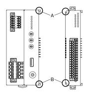
Confirm that the locking clamps of the I/O module are set. Insert the module in parallel to the next one while aligning the grooves of both modules (A & B in the above figure).
