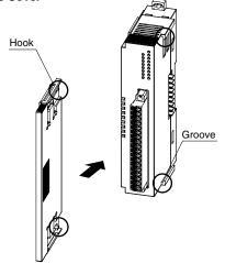
The protective cover is to be attached over the connected I/O module at the right end.
