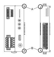
Confirm that the locking clamps of the I/O module are set.
