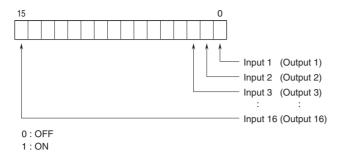
For I/O mixed modules shown below, interlock status is assigned to input 1 (to 3) in addition to output 1 to 16.
