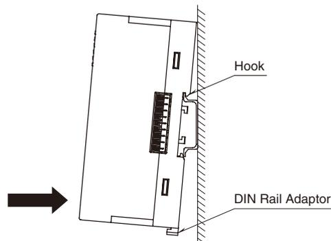
Hang the upper hook at the rear on the DIN rail and push in the lower. When removing the module, push down the DIN rail adaptor utilizing a minus screwdriver and pull.
