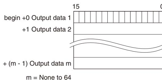
R8-ND2 automatically determines IN/OUT area size of DeviceNet when the power is turned on according to the configuration of the connected I/O module.
