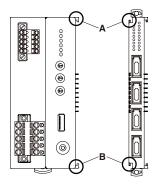
Confirm that the locking clamps of the I/O module are set. Insert the module in parallel to the next one while aligning the grooves of both modules (A & B in the above figure). Maintain it perpendicularly to the rail.
